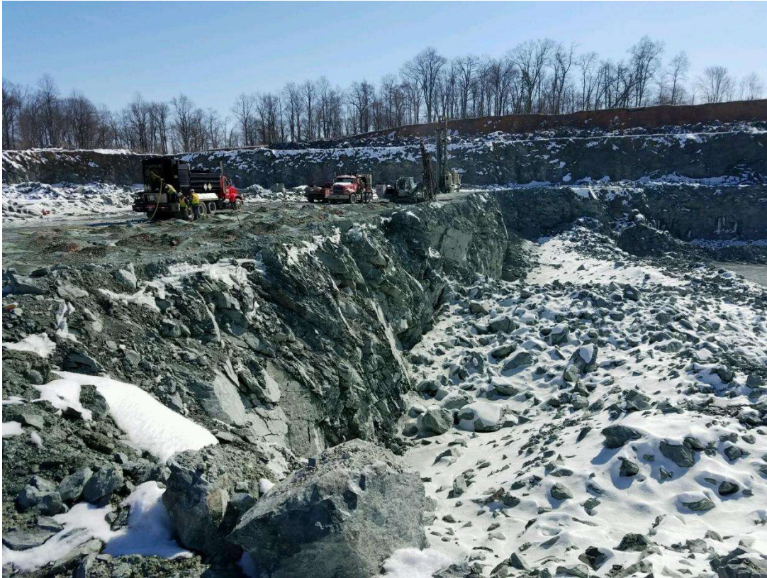
Figure 4 - A typical basalt surface mine with drills and a bulk explosives truck on the bench. Note the level benches and straight highwalls. These features enhance safety and accessibility. Image provided by the author.
